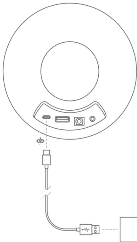
Connect the USB cable to the plug and to the micro USB port on the EUPHO E3.
